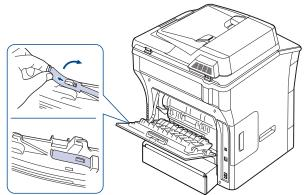
6. Unfold the duplex guide fully.
